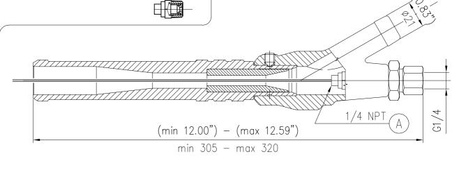
WARNING: Using a regular nozzle NOT suitable to operate at high pressure will produce premature wear and will cause damages on the internal section of the sand blaster.
